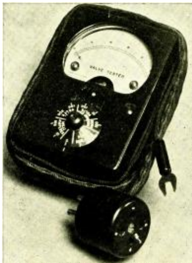
Single-meter test unit made by Ferranti.
